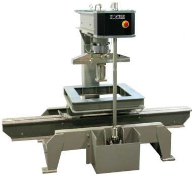
Testing FRC square slab on 300 kN flexure frame to EN Standard
